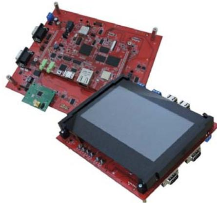
The AM437x PoM and Application Board comes integrated with U-Boot, Linux SDK (3.12), Android Kitkat (4.4.4) and demo applications. The PoM and Application Board can be used to build Video Door Phones, Control Panel, Industrial HMI and PLC, Barcode scanners, Portable Data Terminals, Non-invasive Medical Electronics and Assistive technology products.
