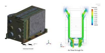
Mistral optimized the design of Chassis Fins to obtain maximum thermal efficiency and avoid over heating conditions that can significantly affect the performance and durability of electronic devices. The custom-built I/O Panel integrated into the Chassis is provided with MIL-C-38999 type Connectors for power and I/O Signals.
