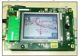
The Navigation Reference Design supports SmartST<sup>™</sup>, navigation software from Navman and has four RF modules: GPS, GSM/GPRS, WLAN and BLUETOOTH on a single small form factor board running Microsoft Windows<sup>®</sup> CE on TI's OMAP5912 processor. The NRD provides product developers with an easy-to-use platform to simulate or test their GPS and wireless applications. This reference design can
