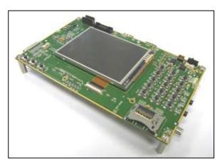
The OSK is designed with a modular and extendable architecture. It is comprised of separate processor and power modules providing reconfiguring flexibility to future processors and power modules. Expansion connectors on the board provide extensibility to a wide range of peripheral interfaces. A key feature of the OSK is the support for an LCD display and DVI to connect to external digital display devices.
