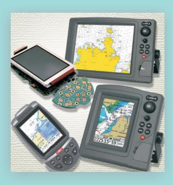
The design needed to be a low-cost device with low-power consumption that used existing application software. It also needed to conform to marine regulatory standards defined in IEC 945.
