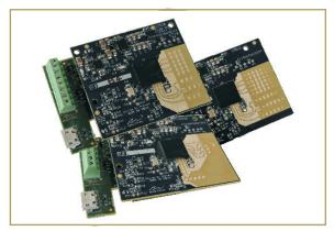
The Automotive RoM operates at frequency bands of 76-81GHz & is ideal for next gen ADAS applications.
