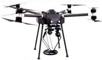
The data from the detection sensors are sent to GCS for geo-tagging the location of the mines. On completion, the detection sensor is replaced with a multi-functional gripping arm for detonation.
